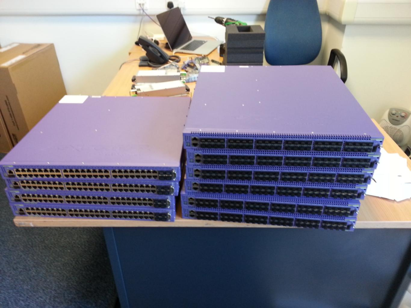
INEX is upgrading to a VPLS network build on Extreme Networks kit
